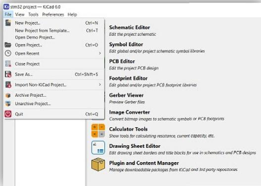
in the top left corner, next click 'New Project' then assign the project a name. We will start out by creating a schematic. To do this we will click on the 'Schematic Editor' icon. To open the blank schematic editor canvas. This board will be based on the STM32F103C8T6 original design.
