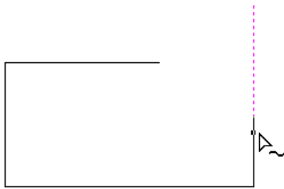
First click creates a preview extension line from the selected vector span.
