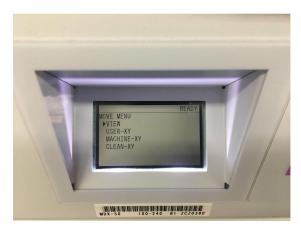
If you want to inspect the piece, Press MENU until you reach the move menu, then go to VIEW this can be used to move the table close to the front.
