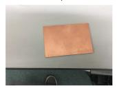
Put the double sided tape on the back of your board, making sure that it doesn't overlap and try not to touch the sticky bit.
