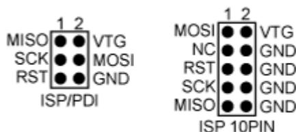
A few ISP programmers are powered by the target power supply. In this way they easily adapt to the correct voltage level of the target board. Other ISP programmers, such as STK600, can alternatively power the target board via the VTG line. In such a case, it is important that the power supply on the target is not switched on.
