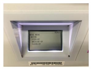
If you want to inspect the piece, Press MENU until you reach the move menu, then go to VIEW this can be used to move the table close to the front.
