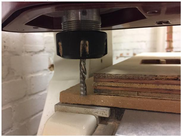
Lift top: set the top limit well above the work surface (about 20mm) which is clearly above the 6mm safe z. Press Enter when done.
