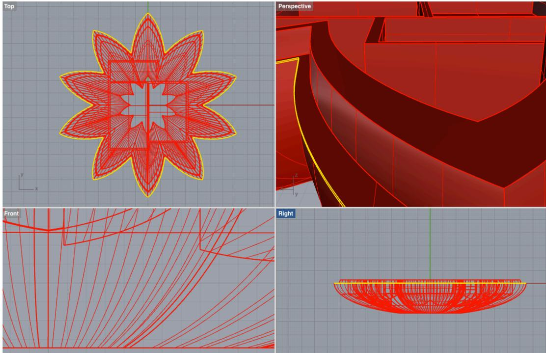
Then select all – Ctrl A and Join. This joins the 3 surfaces into one open polysurface.
