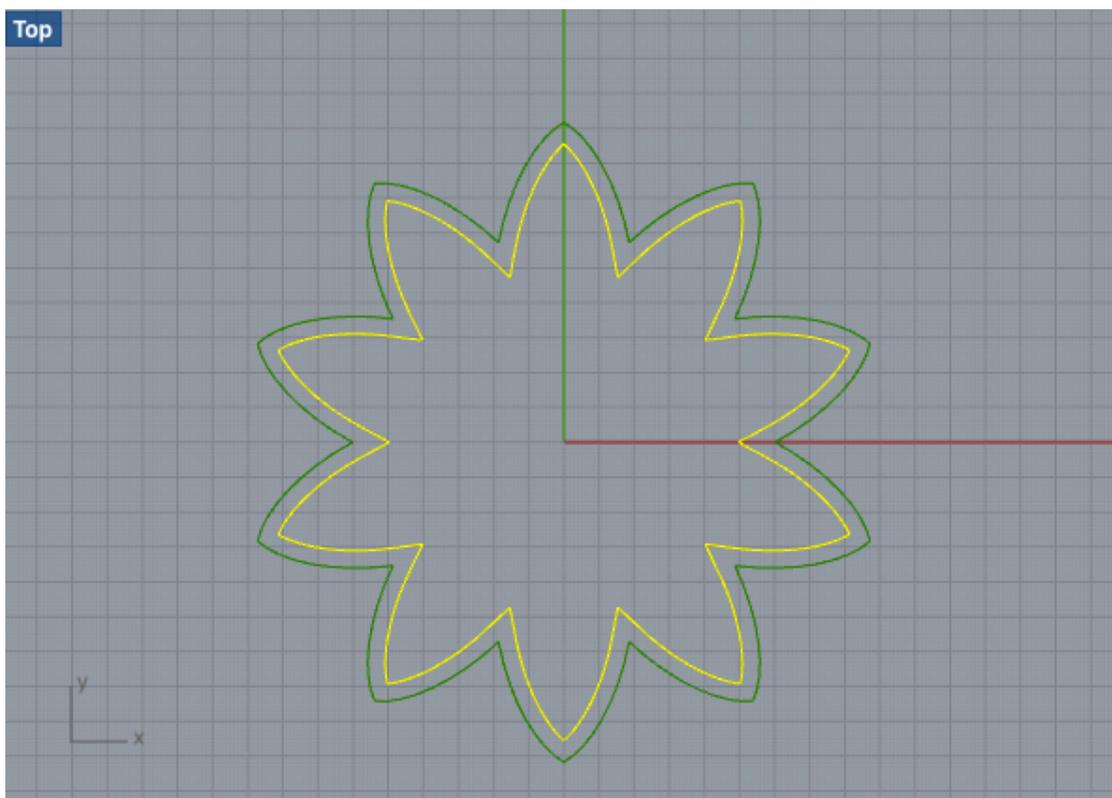
Next, the curves for creating a revolved shape (walls) were offset for thickness by 5 mm:
