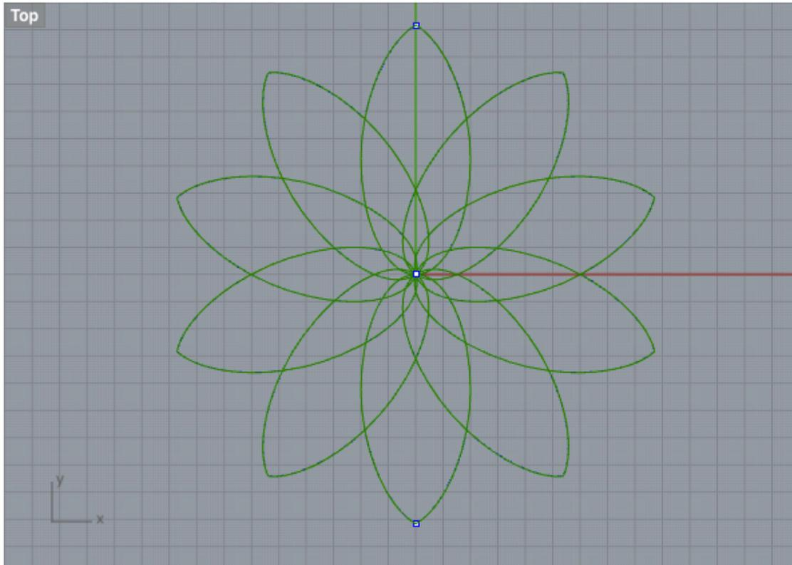
These lines were duplicated to create 2 sets for working separately on the the 2 halves of the flower form. On the top part a Curve Boolean operation was carried out to create a cut-out form in the centre of the shape to let the light in:
