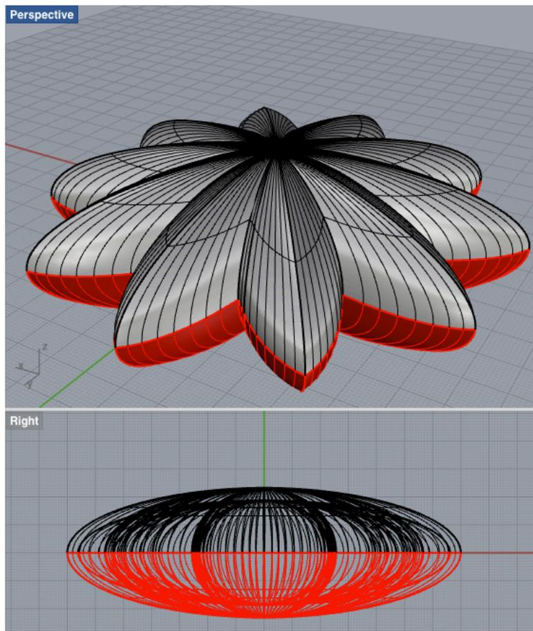
... and a flat surface was made by a Boolean operation, for the bottom part to make it stable.
