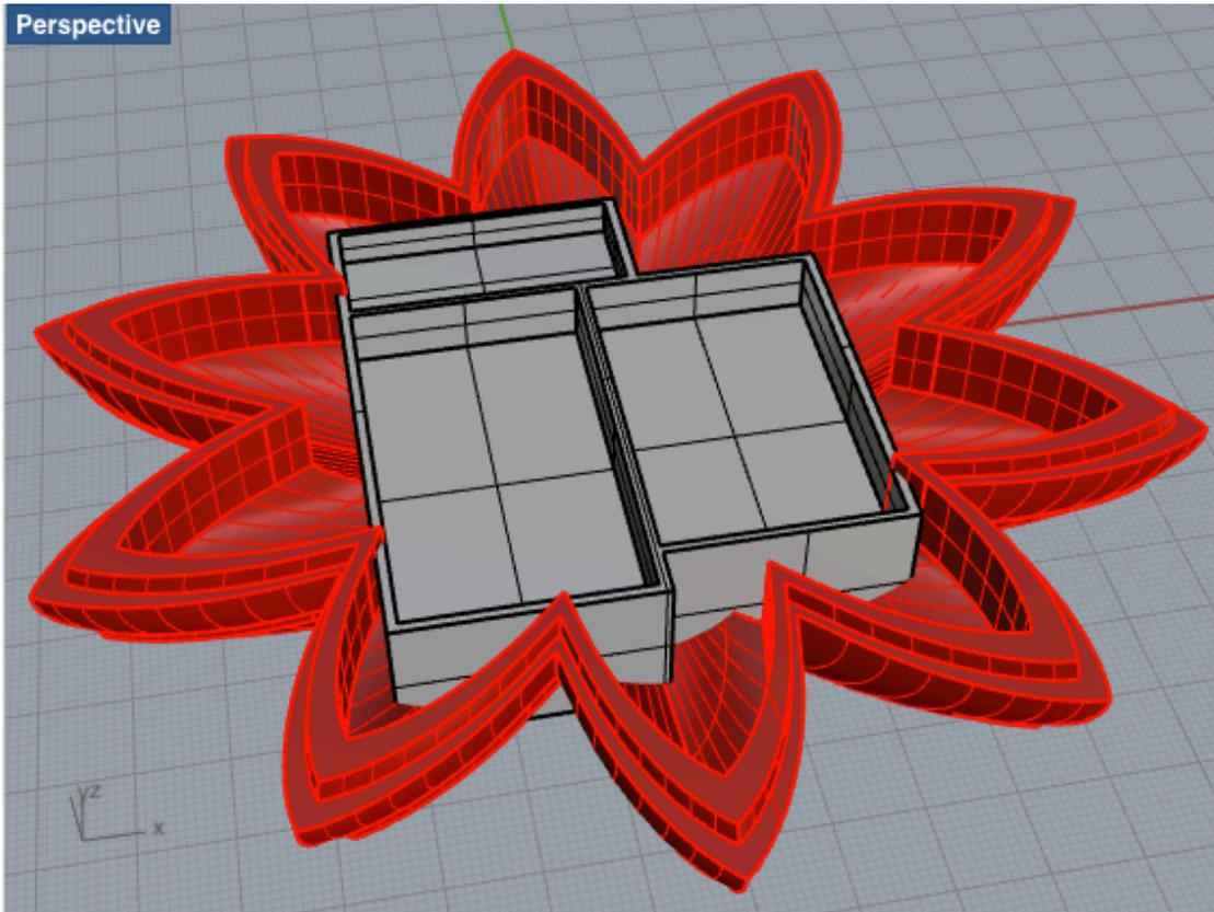
The boxes were then trimmed to fit snugly into the bottom shape.
