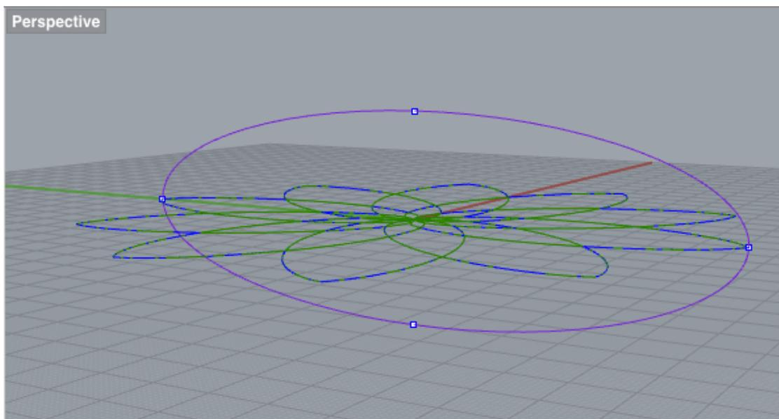
The outer lines of the flower shape were offset to create the wall thickness ( 5 and 3 mm) for the bottom and top parts:
