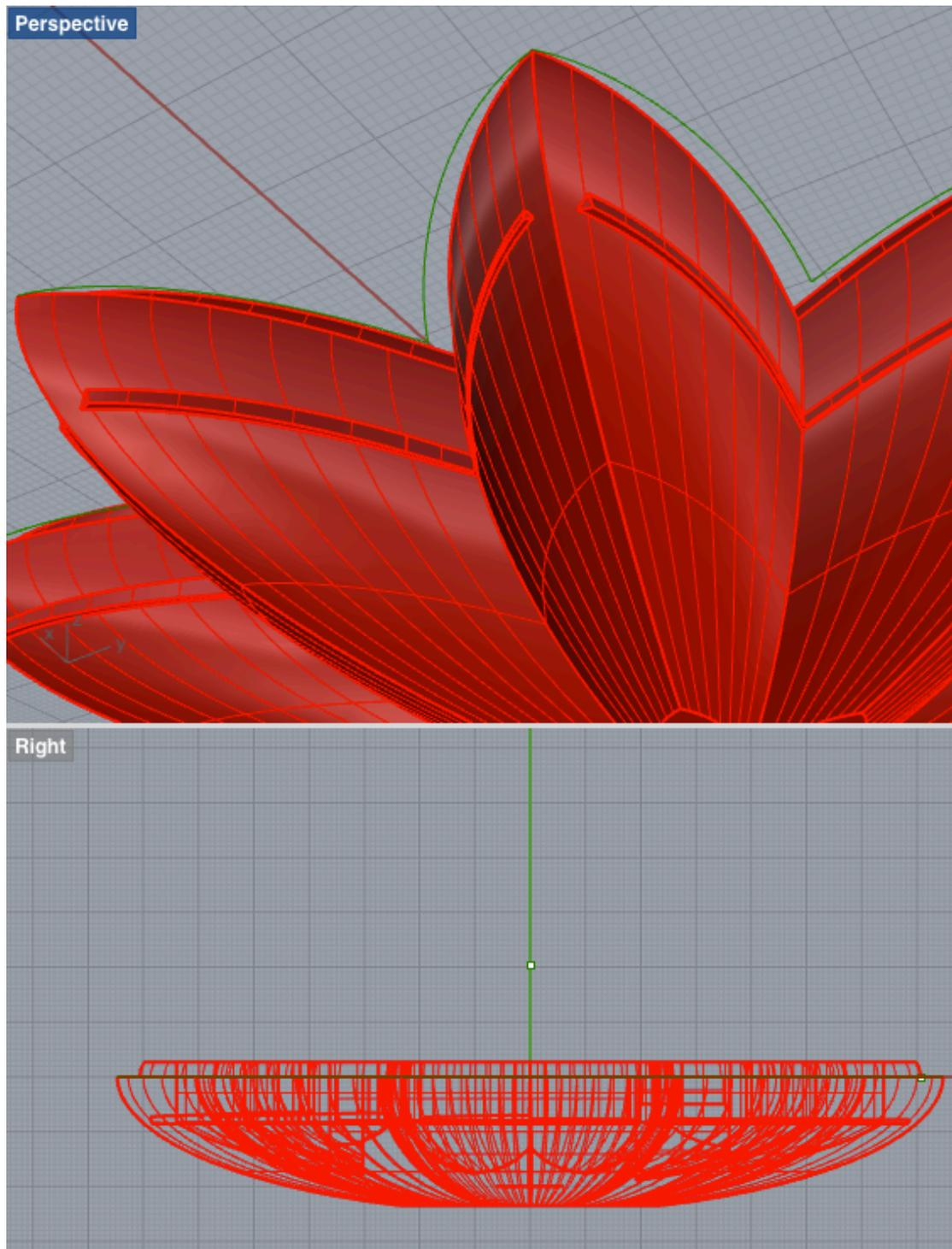
Various actions/commands were tried to remedy this, such as extruding surfaces, deleting the bits standing out and trying to patch the holes. What worked in the end was to delete the holes that were inside a plane, then using untrim surface and cutting the surfaces again to the right size.
