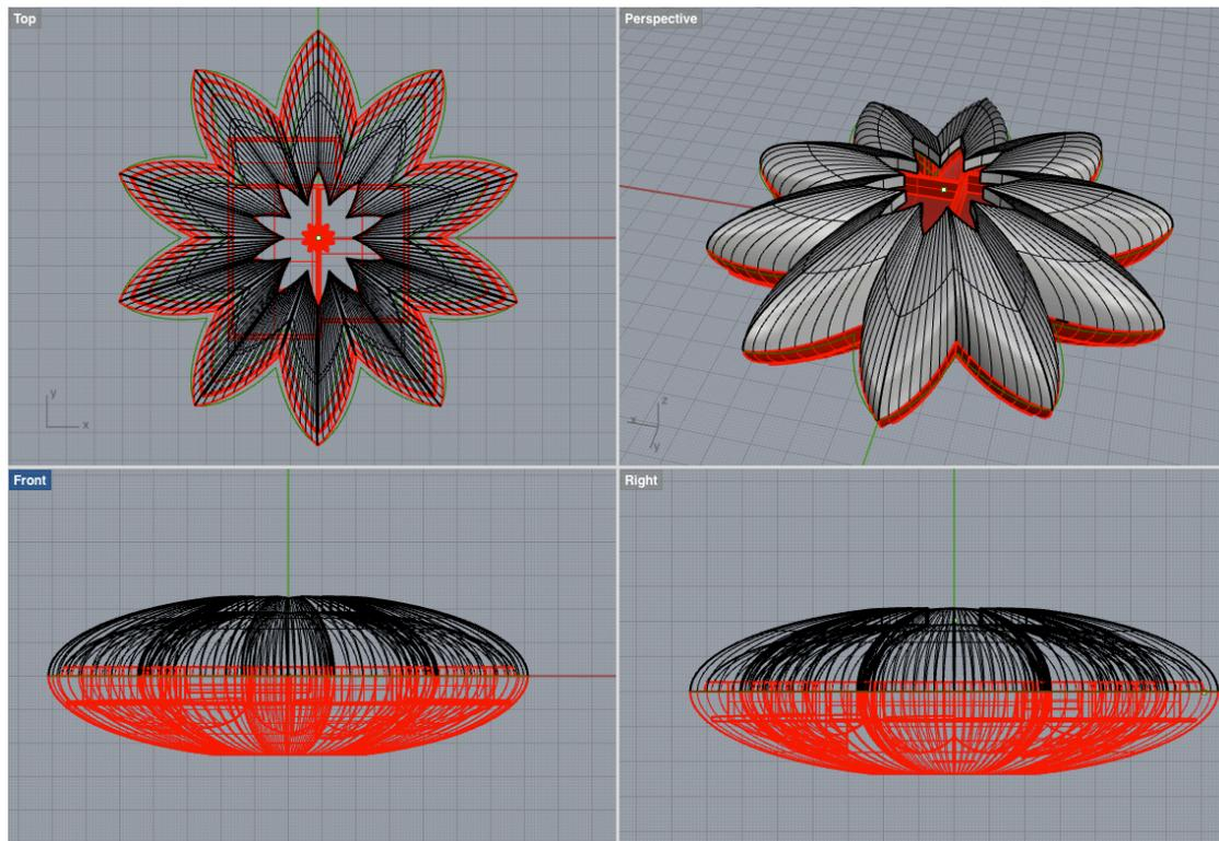
On a closer inspection of a model it turned out that I had made a mistake in a Boolean Union action, with the result that bits were sticking out of the bottom part of the model.
