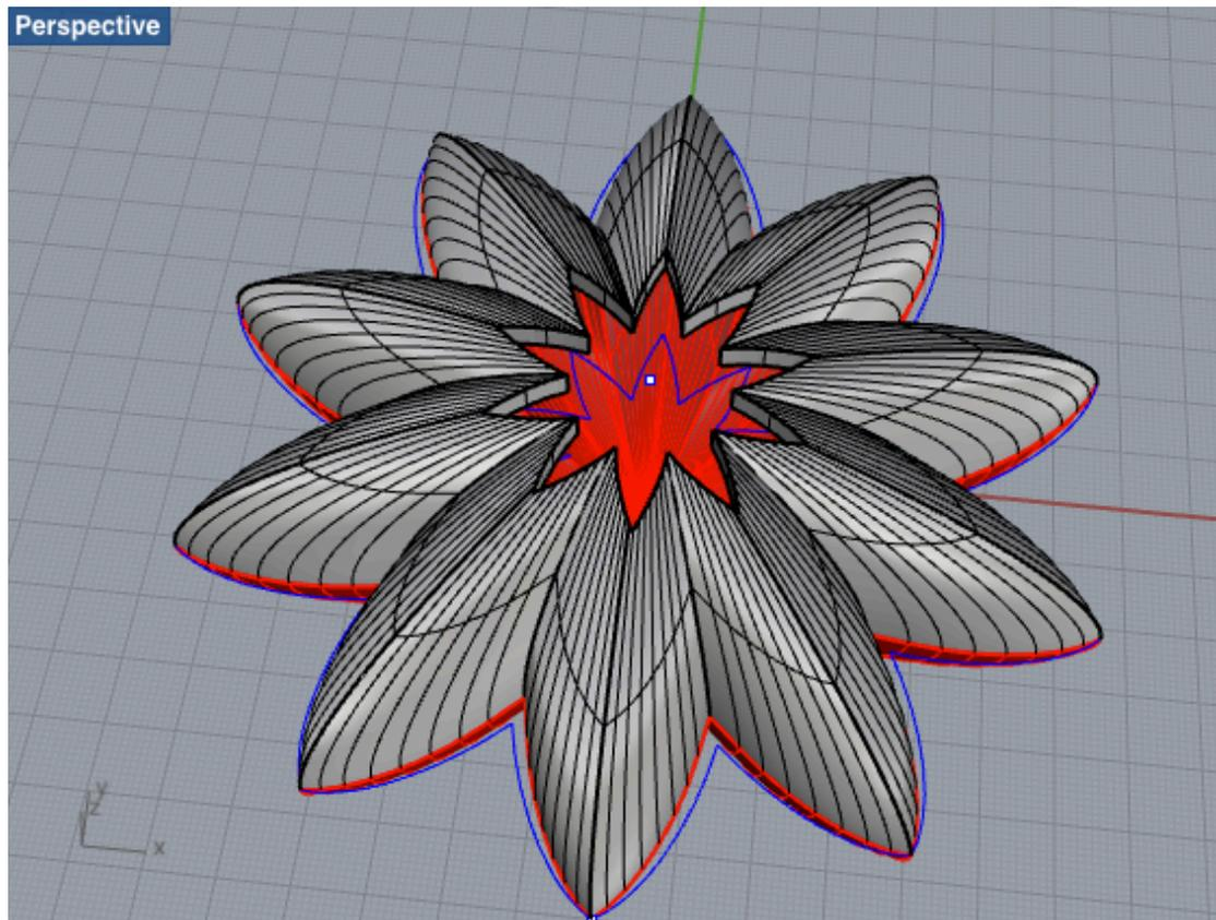
The bottom part now required an extra ridge to be added on the inside of the rim. This was created from curves of the edge.
