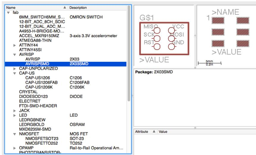
Connector (allowing the board to be programmed, through a cable)
